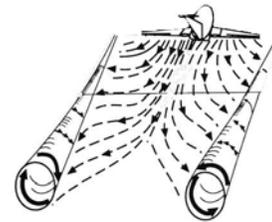
By breaking up vortices, winglets reduce the drag on an airplane, which translates into fuel savings. Conventional upright winglets are currently used on a number of airliners, including the Boeing 747-400 and the Airbus A330 and A340. On some of its 737 models, Boeing uses "blended" winglets, which curve up from the wing instead of sticking straight up.
