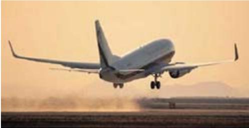
Among the other important contributions made by NASA's Dr. Whitcomb are winglets (first used on Learjet). A winglet's purpose is to reduce turbulence at the tips of an airplane's wings. The air pressure on the bottom of a wing is greater than the pressure on top, so when air flowing across the two surfaces meets at the wingtip, it forms a vortex—a miniature tornado.
